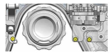
Insert new rubber tips of 17430UK to the rear housing as shown. The rubber tip for REC actuator should be inserted to upper hole as shown.
