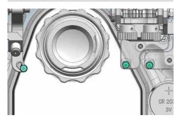
Remove three original rubber tips from 17430 NA-a1 rear housing as shown.
